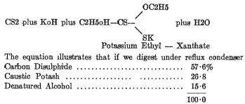
we should upon the completion of the reaction obtained crystaline Potassium xanthate which, however, is soluble in alcohol and can be employed at any strength to effect flotation of copper salts.
